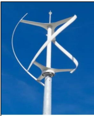
Figure 7: Vertical Axis Wind Turbine
